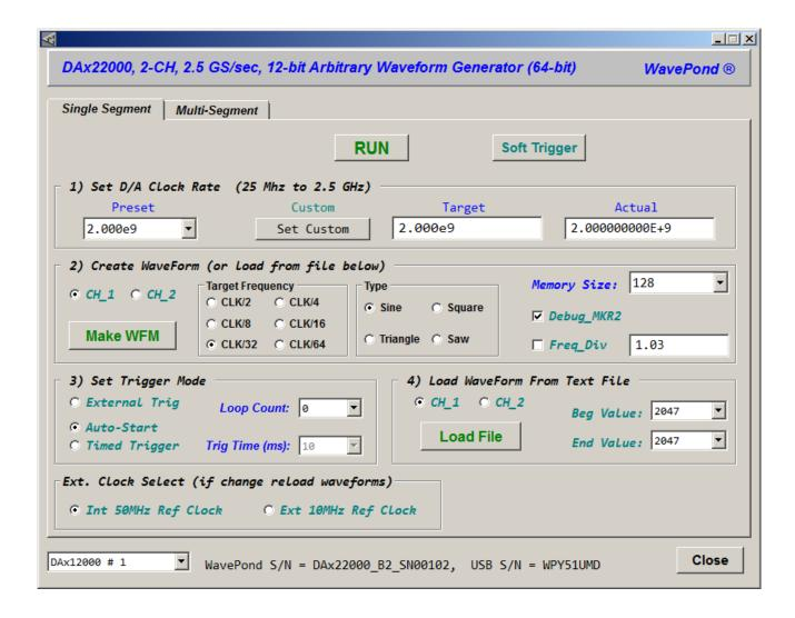
Use "dax22000\_GUI\_xx.exe" GUI to verify drivers are installed correctly and to load simple sine and custom waveforms. (xx = 32 or 64)
